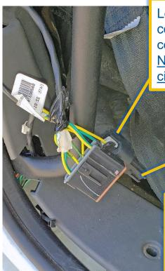
Locate the terminating resistor connector beneath the seatbelt cover behind the driver's seat.
