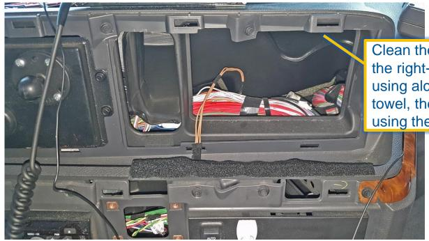
Clean the top of the duct behind the right-center dash panel using alcohol and a paper towel, then mount the antenna using the tape provided.
