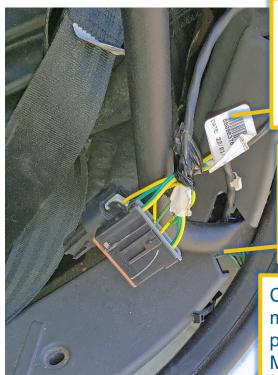
Locate the terminating resistor connector beneath the seatbelt cover behind the driver's seat.
