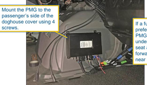
If a fully hidden install is preferred, mount the PMG inside the box under the passenger's seat and route the cables forward under the carpet near the kick plate.
