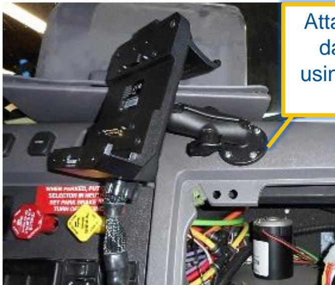
Attach the RAM mount to the dash above the glove-box using bolts and large washers or a backing plate.
