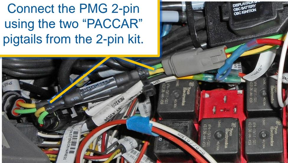
If the vehicle connector comes apart showing 4 pins and a resistor, remove that piece from the black 2-pin and reinsert it in the blue female connector.
