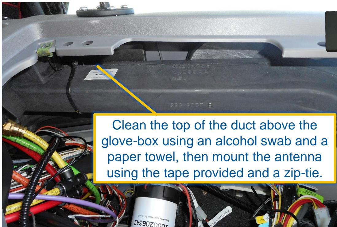
Clean the top of the duct above the glove-box using an alcohol swab and a paper towel, then mount the antenna using the tape provided and a zip-tie.
