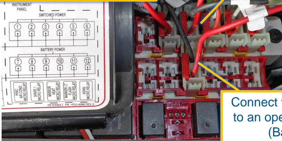
Connect the Constant Power plug to an open spare port on the rear (Battery Power) row.
