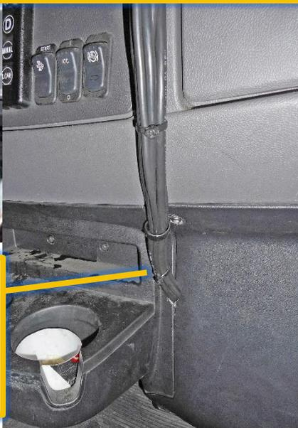
Notch the panel below the glove-box and route the cable into the dash.
