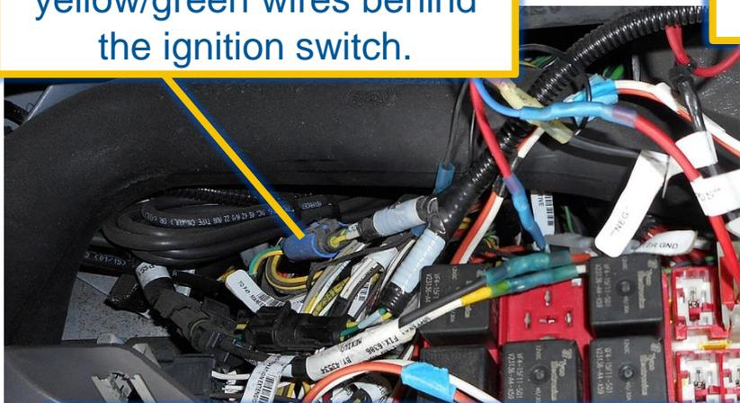
Connect the PMG 2-pin using the two "PACCAR" pigtails from the 2-pin kit.
