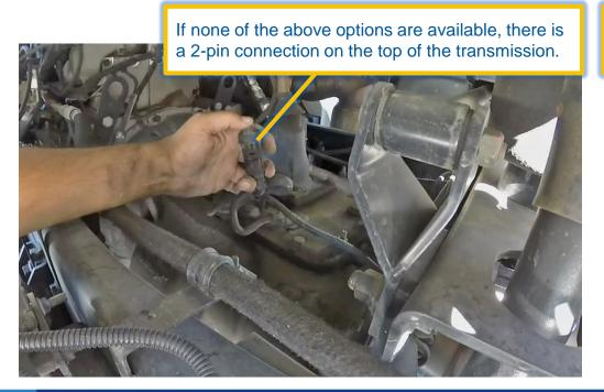
Due to cable length limits, accessing the transmission point may require purchase of 2 J1939 extension cables, part L-016-0628.
