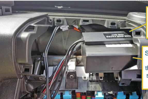
Attach the Antenna to the PMG using the tape provided.
