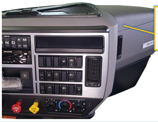
Remove the passenger dash panel. Clean the top of the airduct using alcohol and a clean paper-towel, then mount the antenna using the tape provided.
